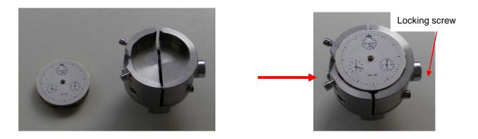
2. Squeeze the movement by turning the locking screw.
