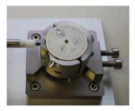
3. Turn the knob in order to adjust the buffer in such a way as to stop the movement of the table right after activating the movement's push-button.
