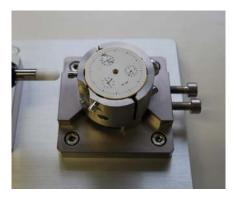
2. Move the mobile table and rest the tip of the sensor against a push-button.
