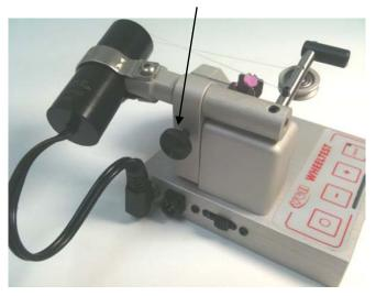
Figure 6: Adjustment of the axial position of the motor
