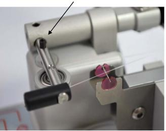
Figure 7: Adjustment of buffer height
