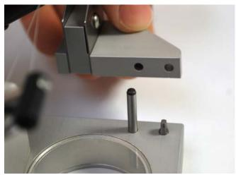
Figure 3: Positioning pins
